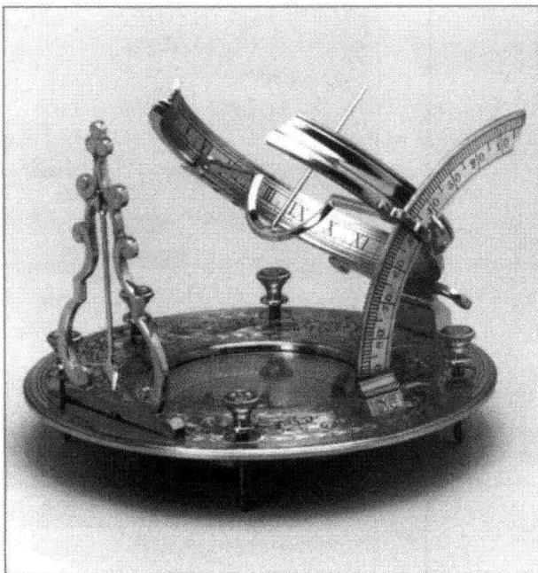
Fig.3. The dial set up for use at 49° N
