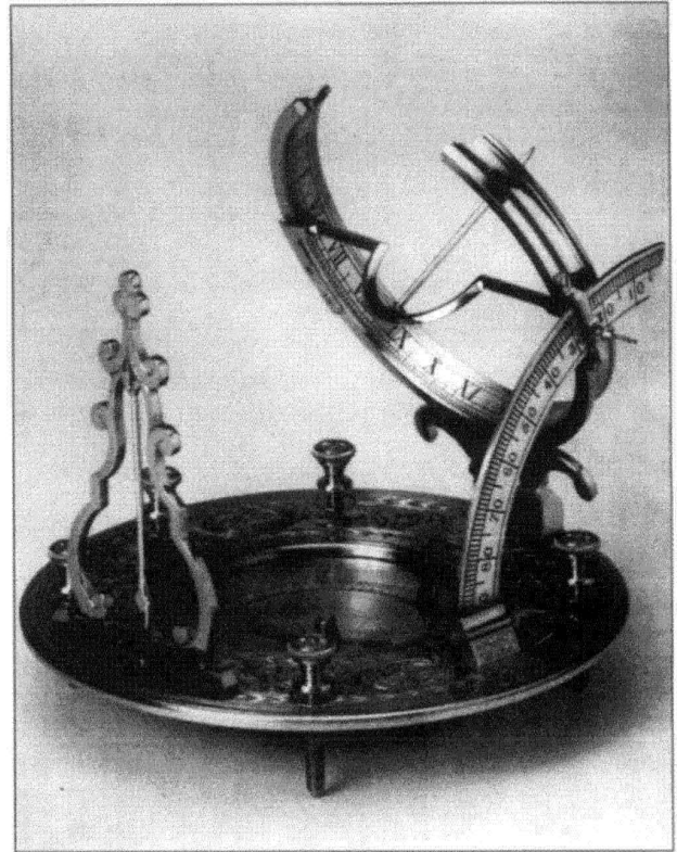
Fig.4. The dial set up for use at 27° N
